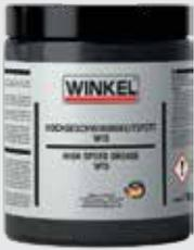
High Speed Grease W15 is a special high speed grease reinforced with EP additives, synthetic base oil and barium complex soap. It exhibits a long-lasting performance, especially in equipment parts operating under wet, variable, impact and vibrating load environment.
