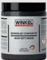
Heavy Duty Grease is a calcium sulfonate complex oil developed specifically for the steel industry. It is formulated to be used for high temperature lubrication of plain and roller bearings exposed to heavy loads in water environments. Its unique thickening structure gives excellent anti-rust properties and outstanding resistance to water washing.
